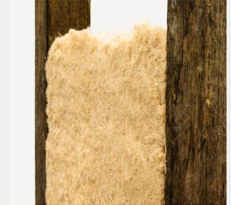
Gutex Thermofibre is a blow in insulation made of two components only: regionally sourced pinewood fiber and ammonium salts which act as a flame retardant. As a result, the product Thermofibre is made from natural, biodegradable materials. It is suitable for stud, rafter and ceiling insulation. It holds a European Natureplus certification that sets strict standards for material health and complies with REACH standards.
